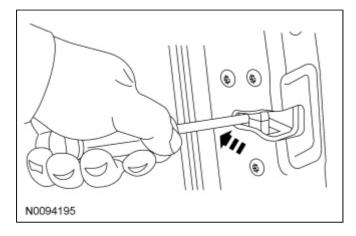
3. Spray the multi-purpose grease into the opening on the door latch for approximately 5 seconds.
